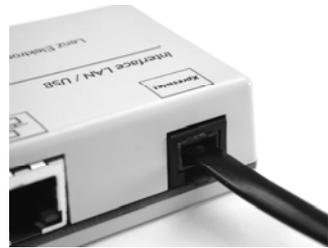
If you want to connect the Interface 23151 to the terminal screws LMAB of a LZ100/LZV100 command station, simply cut the cable in the middle and connect the cable wires to the corresponding terminal screws. The pin assignment is shown in the illustration on the right.
