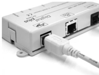
Plug the USB "A" plug into the free USB port of the PC.
